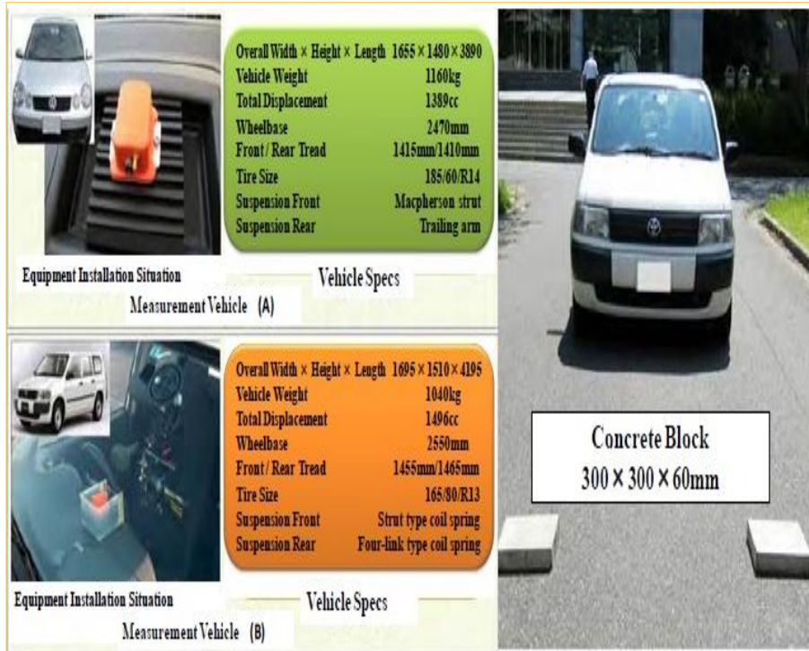
Fig. 10. Spec of measurement vehicle and installation condition of the system
